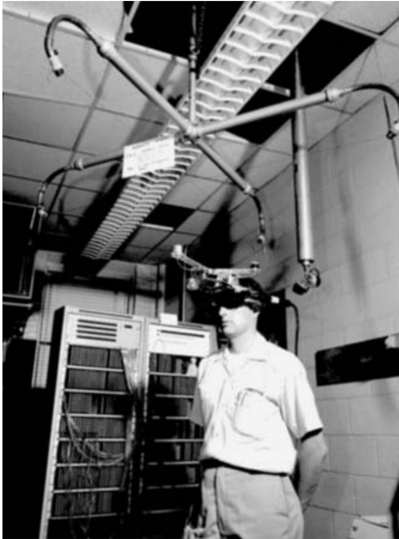
Figure 2.3: Sutherland with his head-mounted display and the mechanical tracker hanging from the ceiling in 1968. Courtesy of wikimedia.org
